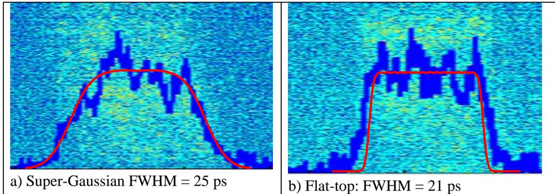
**FIGURE 3.** Streak camera measurement of output pulses.
