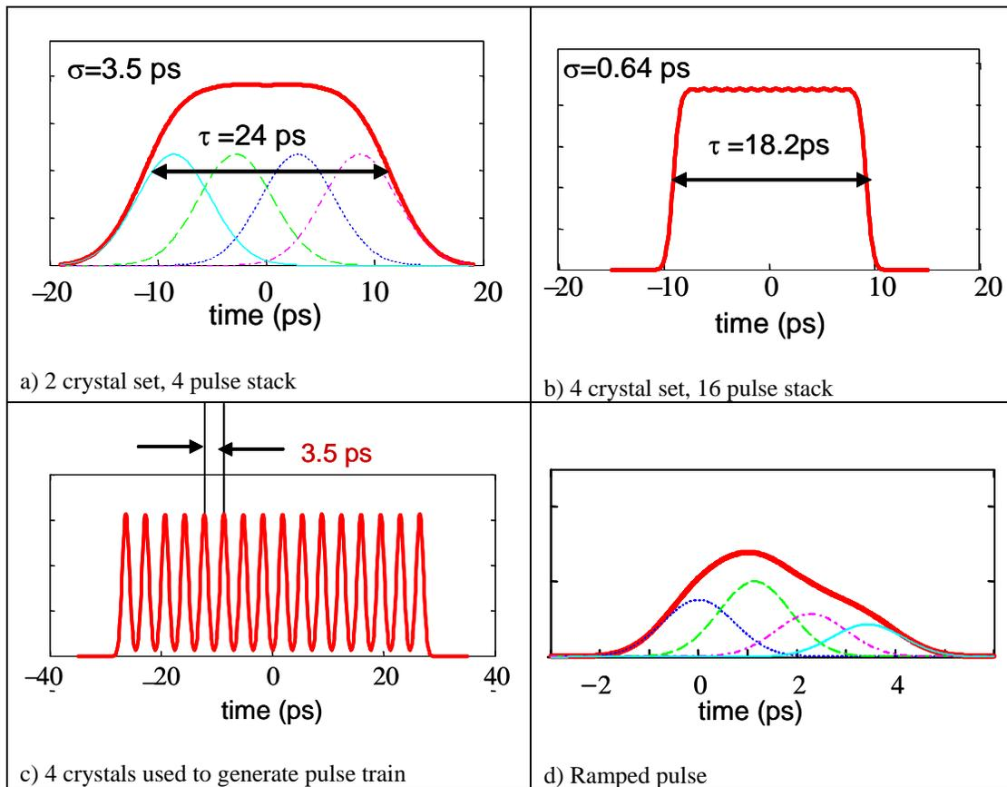
**FIGURE 2.** Output pulses that can be generated with an  $\alpha$ -BBO-based TPS.
